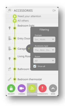
If all installed accessories must be seen, including sensors, then click on the filter tab on the right side of the screen, and check the "Show All" check box.
